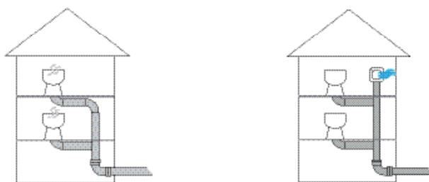
Ventilation is installed with ARIO.
