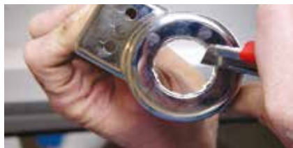
2. Install the AAV with technical gasket
