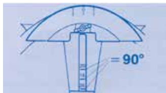
Phase 3 - Use the lever of the clamp until you reach the desired bending angle.
