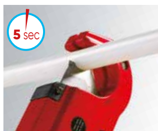
1- Cutting the pipe
